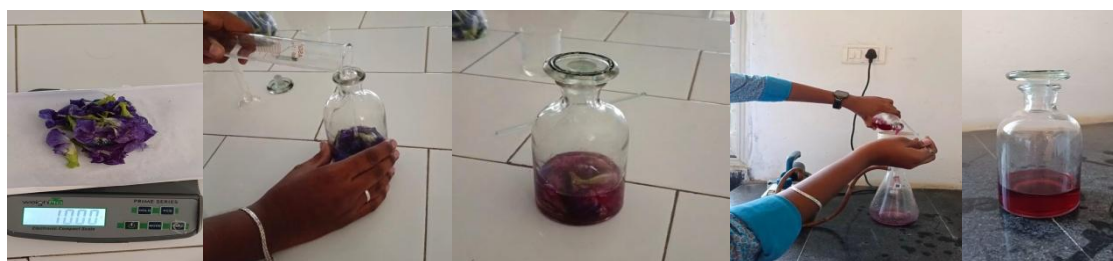
Weighing Addition Of Solvent Maceration Vacuum Filtration Prepared Extract
