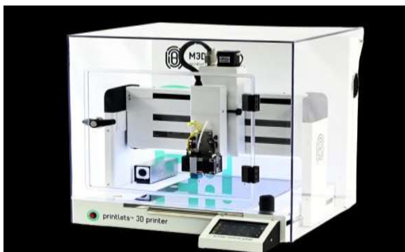
Fig 6: A 3D printer used for fabricating pharmaceutical products, enabling precision drug manufacturing
