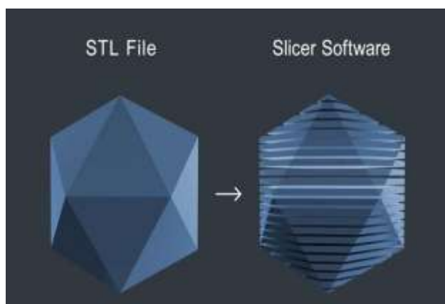
Fig: 2 the process of converting an STL file into sliced model using slicer software
