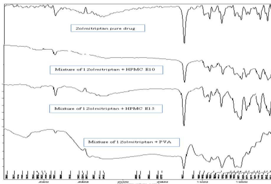
**Figure 2:** FT-IR spectra of pure drug and mixture of pure drug and pure drug with polymer
