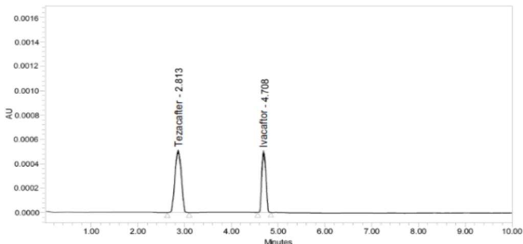
Fig.2(b) : Chromatogram of Tezacaftor, Ivacaftor showing LOQ
