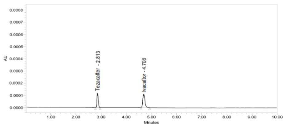
Fig.2(a) : Chromatogram of Tezacaftor, Ivacaftor showing LOD
