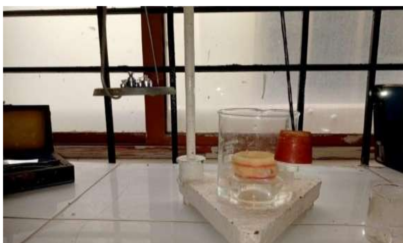
Fig. 2: Modified balance to measure ex vivo bio adhesive strength
