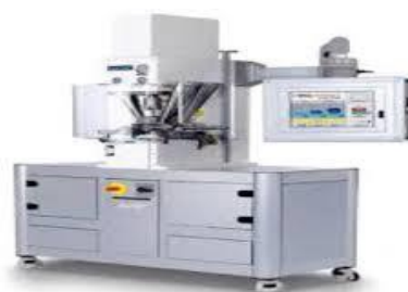
Figure 4 Bilayer tablet press with displacement monitoring [38]
