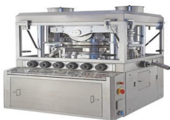
Figure 3 Double sided tablet press [37]
