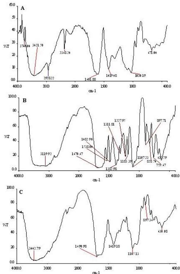
Figure 2. FT-IR Spectras of sodium alginate(A), Acyclovir(B) and drug loaded alginate beads(C)
