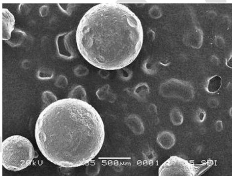
**Figure 1: SEM image of floating Alginate beads**
