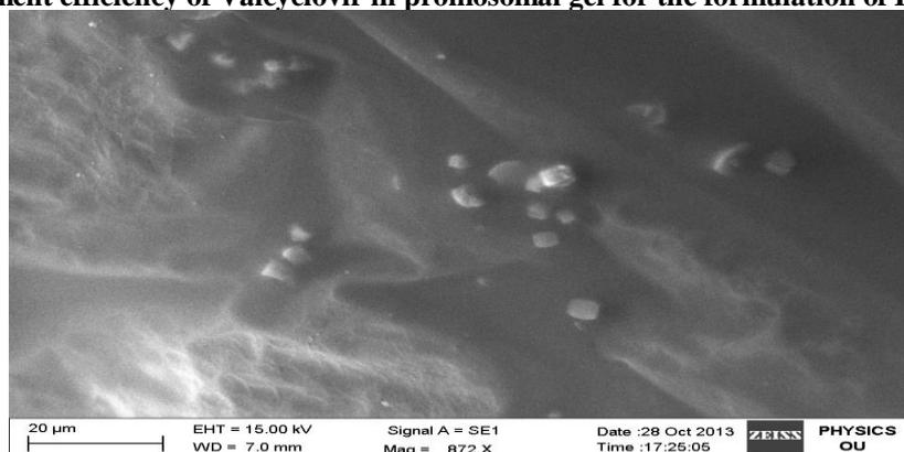
**Fig. 2: Scanning electron image of hydrated F1 proniosomal formulation**
