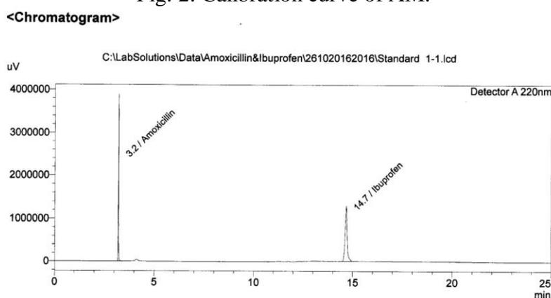
Fig. 3: Chromatogram of standard concentration (0.1 mg/ml AM+0.1 mg/ml)
